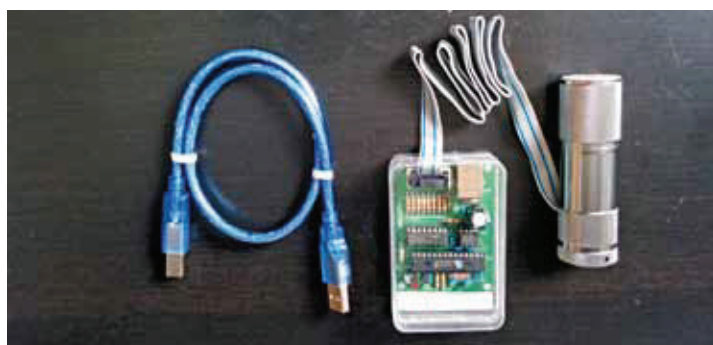
The Jena electronic tongue ("Multiionen-Sensoricard") is composed of a measuring head with ten electrodes for eight measurement channels to determine the vector components, an electronic unit, a USB cable and a computer
