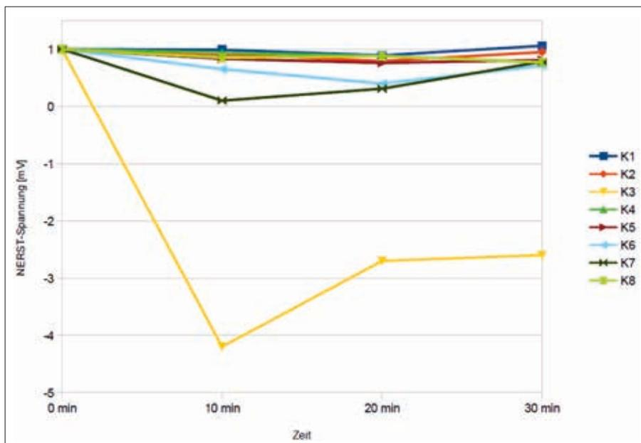
Fig. 3: Chronological sequence of voltage values of the Jena Electronic Tongue measuring a wine after opening the bottle and pouring the wine into a wine glass. Measuring device Card 270, Tongue 206, measuring head 3M1
