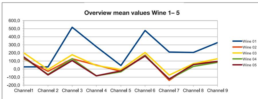
Fig. 1: Results of five wine varieties recorded with the Jena Electronic Tongue Multi-SENSORICCARD® in a 9-channel configuration
