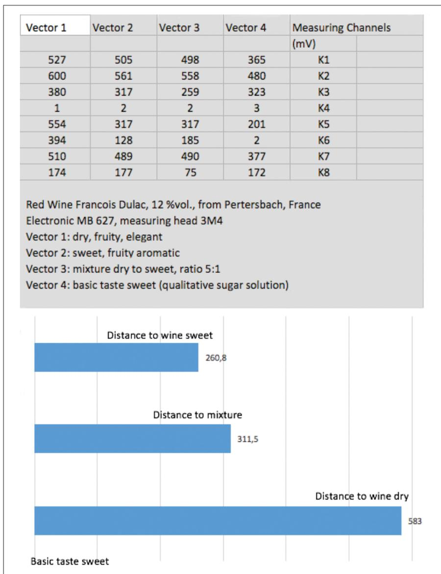
Fig. 4: Example of a solely technical taste description using the Jena Electronic Tongue Multiion-SENSORICCARD®
